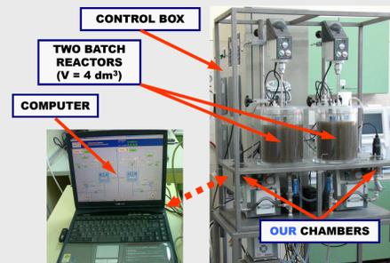
Figure 3 – Laboratory apparatus for conducting the kinetic studies
